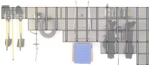
For outside InstallStrips it is best to not center them on the wall stud. Instead you will want to offset the InstallStrip by 0.25" from the center of the stud towards the inside of the panels. This will provide for the best hidden system.
